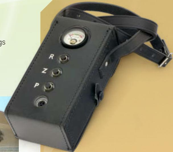
The GRIP Geophone String Analyzer is a hand-held unit, allowing a quick and efficient method of checking Geophone string Resistance, Impedance, and Polarity (GRIP). It is calibrated to match string parameters by a plug-in module, and any deviation from the nominal values are displayed on a panel meter. The unit is temperature compensated and has an audible tone for polarity and low battery warning.
